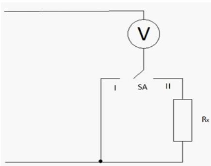
a)  $R_x = \frac{U_1}{U_2} R_v$     б)  $R_x = \left(\frac{U_1 - U_2}{U_2}\right) R_v$     в)  $R_x = \left(\frac{U_1}{U_2} + 1\right) R_v$     г)  $R_x = \left(\frac{U_2}{U_1} + 1\right) R_v$
