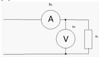
$$\text{a) } R_x = \frac{U}{I} \quad \text{б) } R_x = \frac{U}{I} - R_A \quad \text{в) } R_x = \frac{U}{I - \frac{U}{R_V}} \quad \text{г) } R_x = \frac{U}{I} - R_V - R_A$$
