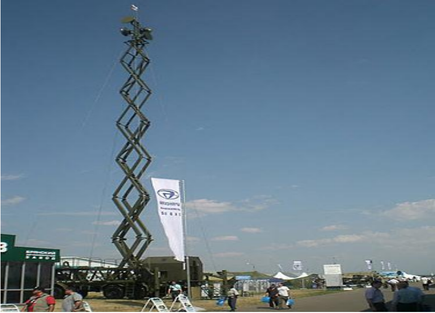
Picture 5 – MIK-MKS Mobile Communications System
